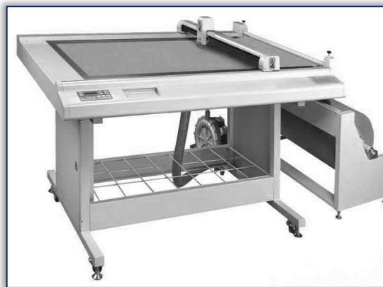
Figure 24 A Flat-bed Plotter
