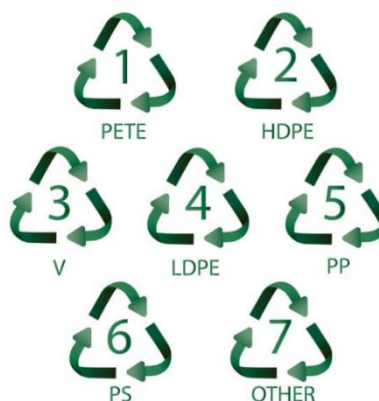
Figure 7: Labeling system of polymers used in different products (LDPE: Low density polyethylene, PS: Polystyrene, for others see text).
