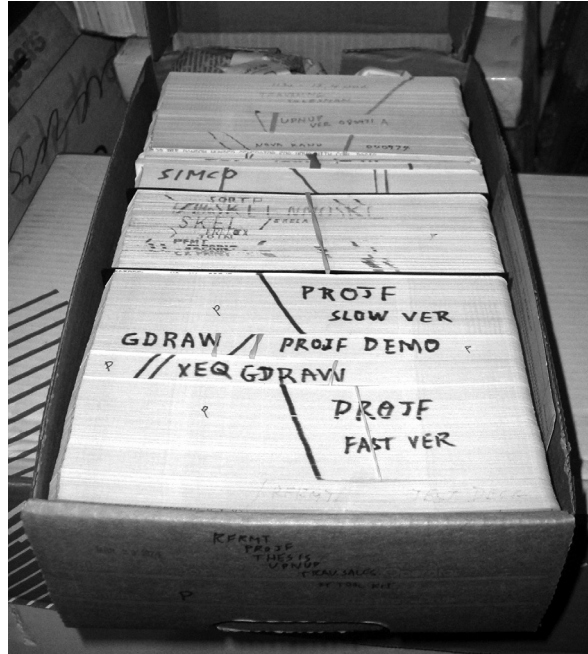
Figure 9.2: Data and Instructions could be Stored on External Punched Cards, Which were Kept in Order and Arranged in Program Decks
