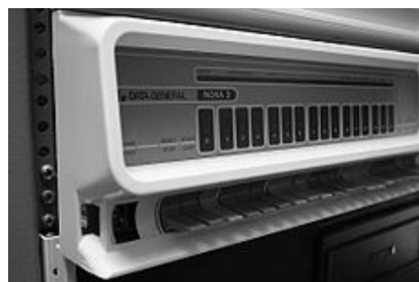
Figure 9.5: Switches for Manual Input on a Data General Nova 3
