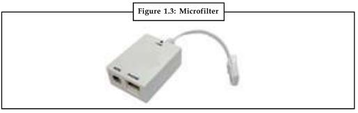
You should have also received a microfilter. This splits the signal in the telephone wire in two: voice and broadband. You plug the dangly end of the microfilter into your telephone socket. Then in the sockets at the other end, you plug in (1) the cable from your own telephone and (2) the cable that came with your router. As these two sockets are different shapes, you can't plug a cable into the wrong socket. Finally, plug in the other end of the router cable into the router itself.
