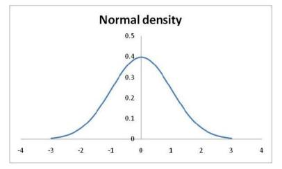
Figure 1: The probability density function of a normal distribution with mean 0 and standard deviation 1.
